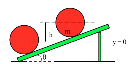
where  $I_p$  is the moment of inertia about the contact point. We determine that using the parallel axis theorem in Part c (it was  $I_{contact pt} = \frac{5}{3}mR^2$ ). This makes the problem look like (next page):
