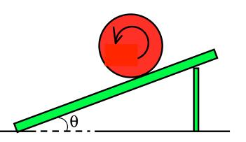
With the angular acceleration term, we now have three unknowns. To get our final equation, we need to remember that the relationship between the <u>angular</u> <u>acceleration</u> about the center of mass and the <u>acceleration</u> of the center of mass is:
