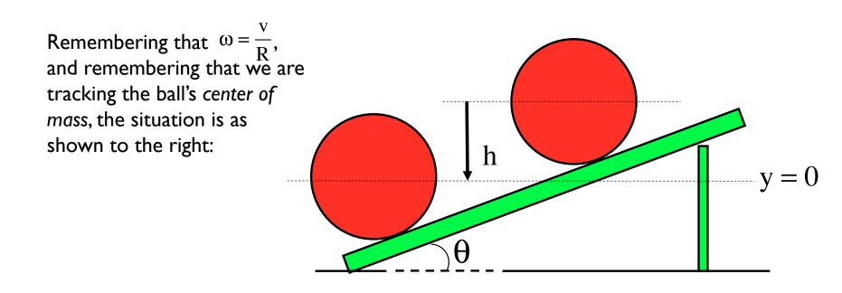
Minor Note: You could have been given the actual distance the ball traveled (i.e., L in the sketch to the right) instead of the ball's vertical drop "h." In that case, you would have had to use the triangle shown to determine "h" (for the gravitational potential energy quantity mgy).
